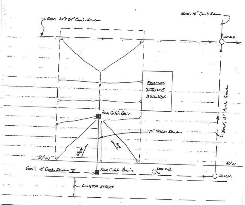
Contractor shall place one (i) or more cotch basins on his proposed lot, the run this collection system into the City system by placing a cotch basin over the existing 12" storm sever along Clintan Street. We would prefer that the Contractor place this Cotch basin on the line where the 4"-6" top is currently located, This system will not eliminate pending or some backup,
