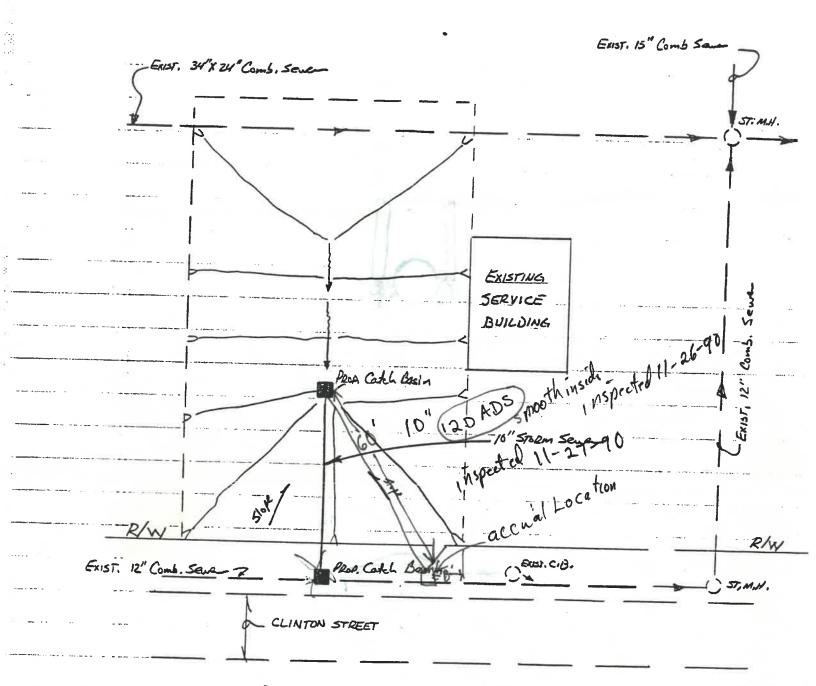
Contractor shall place one (i) or more catch basins on his proposed lot, then run this collection system into the CKY system by placing a catch basin over the existing 12" storm sever along Clintan Street. We would prefer that the Contractor place this Catch basin on the line where the 4"-6" tap is currently located, This system will not eliminate pincling or some backup.
